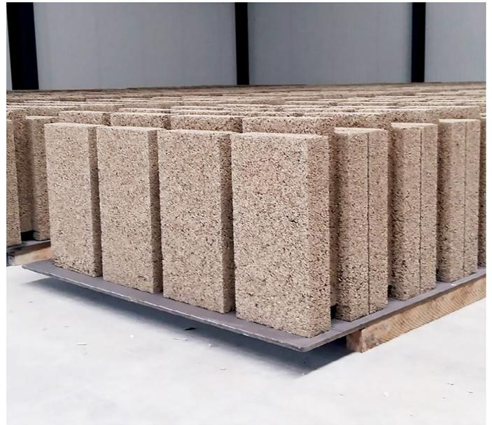
The industrial processes at the HempBLOCK manufacturing facility are specifically designed for the production of hempcrete blocks. Annually the factory produces more than 70,000 blocks.
